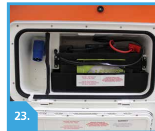
23. CHECK LEISURE BATTERY IS SECURE & BATTERY BOX IS LOCKED
