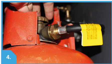
4. OPEN THE VALVE ON THE BOTTLE
