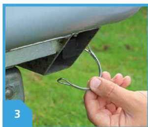
3 REMOVE THE D-PIN TO RELEASE LEG
