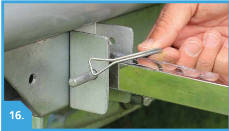
REMOVE THE FOUR BED SUPPORT LEGS
