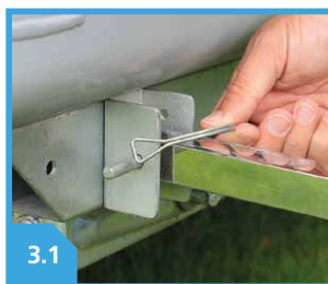
3.1 SECURE BASE OF LEG WITH D-PIN
