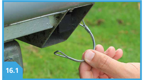
D-PIN SECURES BED SUPPORTS
